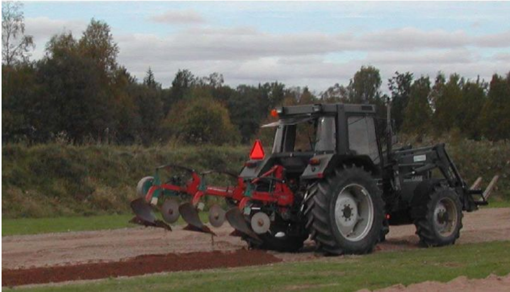
Figure 2: Preparation of standard test lanes – loosening the soil Picture © SWEDEC
