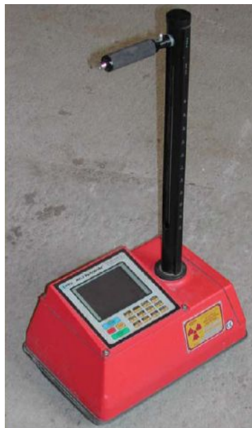
Figure 5: CPN International Model MC-3 Portaprobe nuclear densimeter used by SWEDEC to monitor soil compaction levels of the standard test lanes. Picture © SWEDEC
