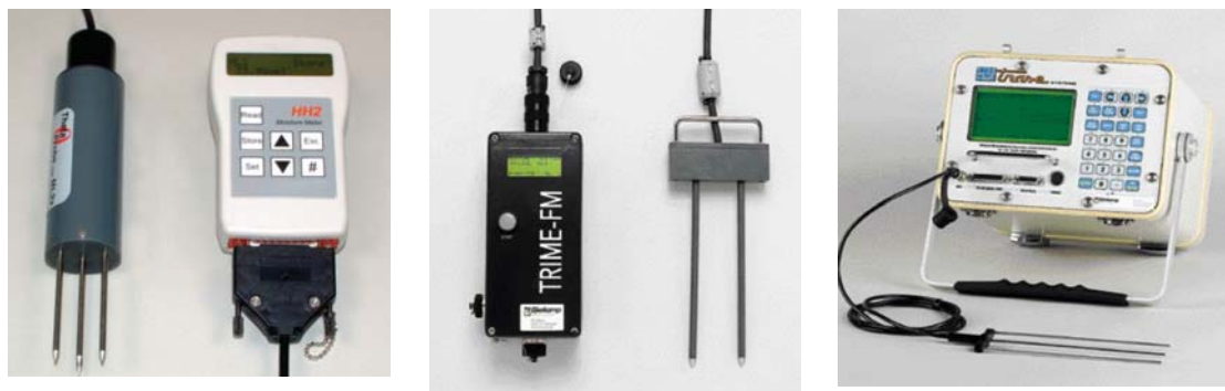
(a) (b) (c) Figure 6: Examples of FDR (a) and TDR systems (b, c) consisting of measuring probe and meter.
